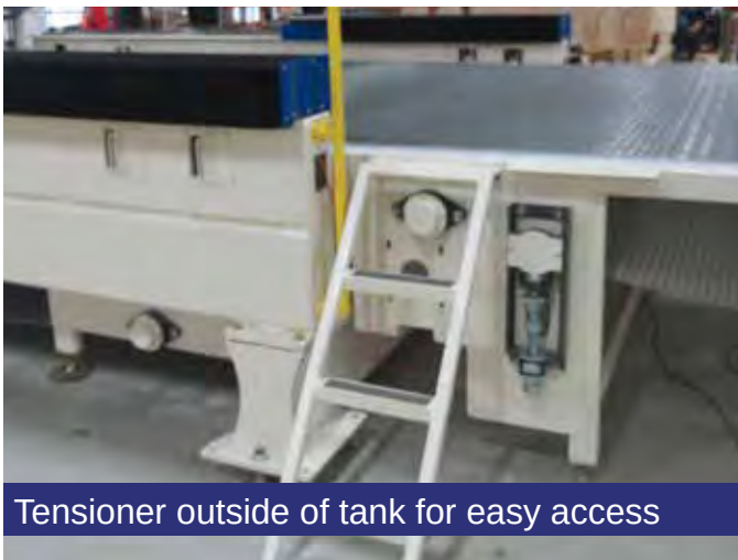
L-3025 waterjet with stainless steel lined tank
