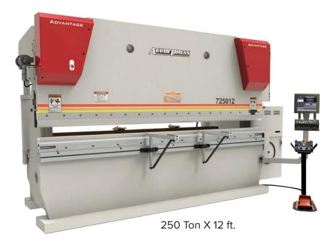
The Advantage Rocker Arm has stood the test of time with thousands of machines shipped all over North America. Offered in a wide range of available sizes from 25 tons to 3000 tons.
