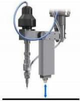
Single Z axis head and nozzle with Auto Height Gage
