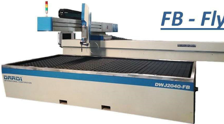
Extremely Stable Cast Iron Bases for all DARDI Flying Bridge Models
