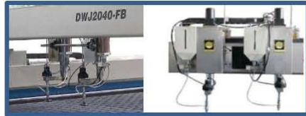
Dual Z axis heads with one nozzles per head
